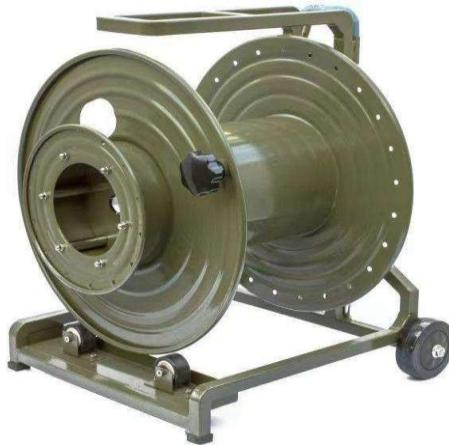
**Product Overview:** The TAC-DRM-RL100 cable reel, manufactured by ANDA TELECOM PRIVATE LIMITED, is a robust and versatile cable management solution designed for heavy-duty applications. It's engineered with durable metal materials, equipped with a pull rod and wheels, and features three gears to allow adjustable winding speed. The reel is ideal for efficiently handling a variety of cable sizes, supporting organized cable storage, transportation, and deployment.
